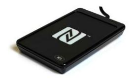
The ACR1252 from ACS is a 13.56 MHz USB contactless smartcard reader that supports ISO 14443 type A and B cards, MIFARE, FeliCa, and ISO 18092-compliant NFC cards and tags. Replacing the popular ACR122U as well as the ACR1251, this reader is equipped with a SAM slot which provides a high-level of security in contactless and NFC transactions.
